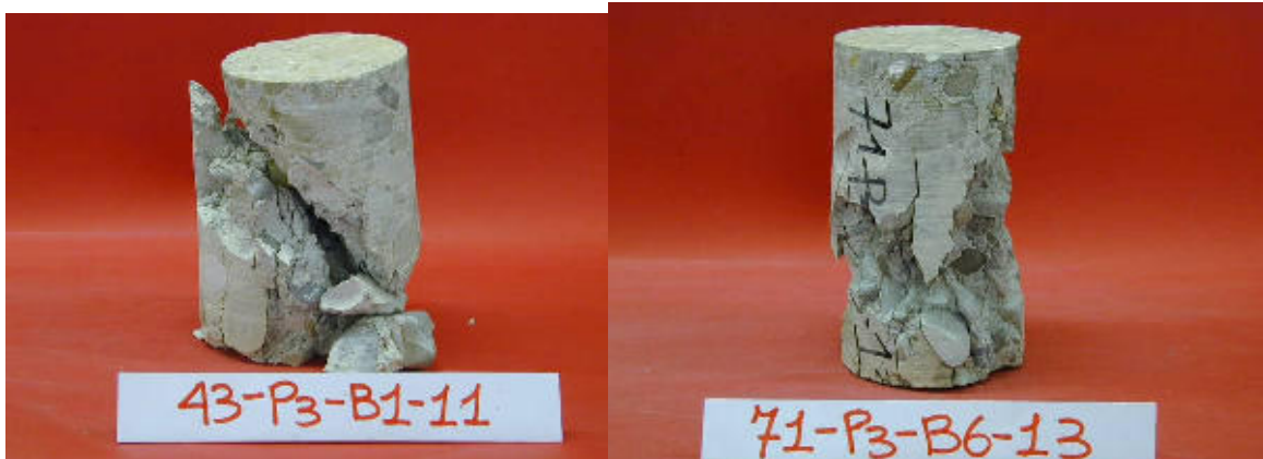
Fig. 12a,b Example of rupture of type “not satisfactory” (on the left) and satisfactory (to right) according to of norm UNI EN 12390-3
